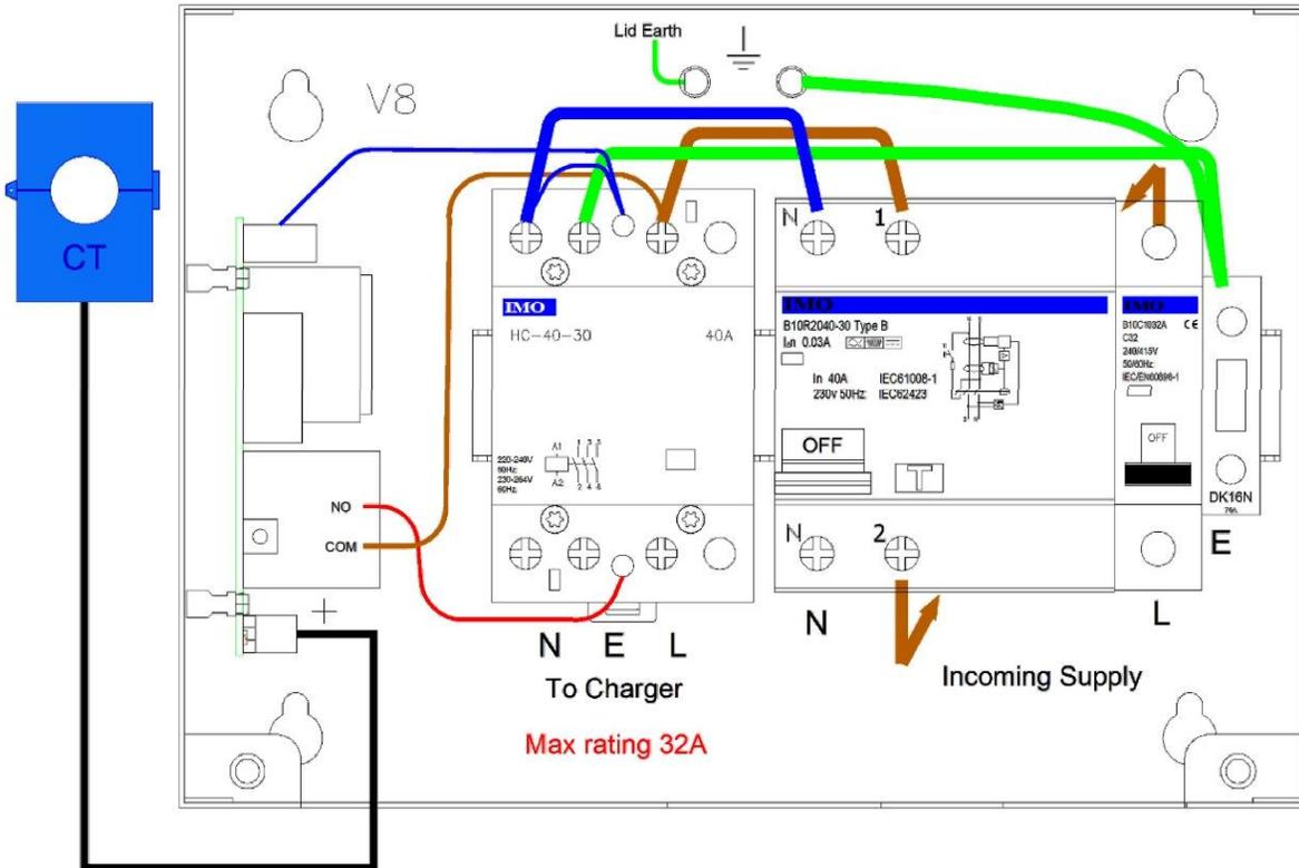
Connect the supply cable from the distribution board (or meter tails) directly to the MCB/RCCD 'Incoming Supply' terminals. Connect the outgoing cable to the contactor L, E & N terminals.
