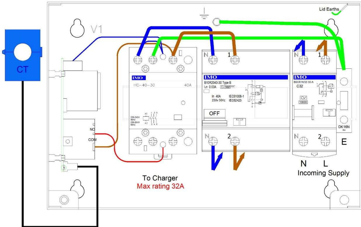
Connect the supply cable from the distribution board (or meter tails) directly to the RCBO 'Incoming Supply' terminals. Connect the outgoing cable to the contactor L, E & N terminals.
