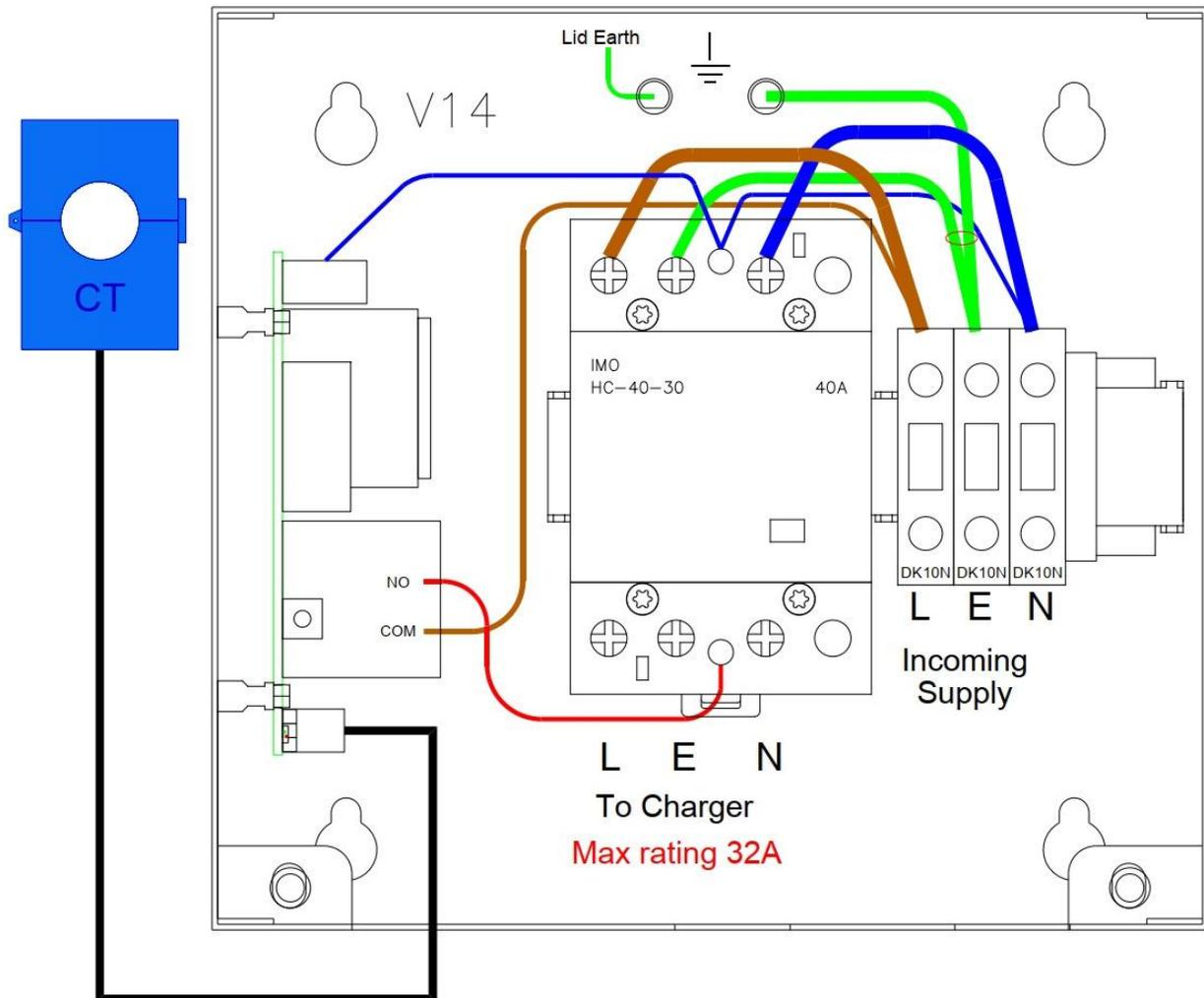
Connect the supply cable from the distribution board directly to the 'Incoming Supply' terminals. Connect the outgoing cable to the contactor L, E & N terminals. If required, connect the CT to the 3 pin connector on the PCB. Check ALL power and earth connections before switching on.
