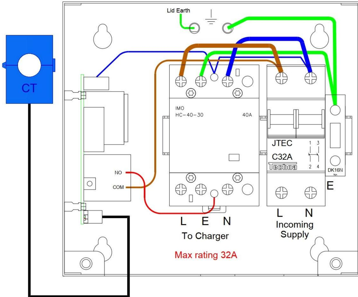
Connect the supply cable from the distribution board directly to the MCB 'Incoming Supply' terminals. Connect the outgoing cable to the contactor L, E & N terminals. If required, connect the CT to the 3 pin connector on the PCB. Check ALL power and earth connections before switching on.
