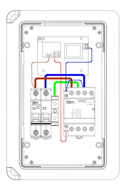
Connect the supply cable from the distribution board (or meter tails) directly to the isolator 'Incoming Supply' terminals. Connect the outgoing cable to the contactor L, E & N terminals. If required, connect the CT to the 3 pin connector on the PCB. Check <u>ALL</u> power and earth connections before switching on.
