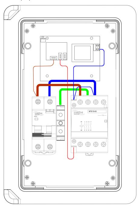
Connect the supply cable from the distribution board directly to the RCBO 'mains in' terminals. Connect the outgoing cable to the contactor N, E, & L terminals. If required, connect the CT to the 3 pin connector on the PCB. Check <u>ALL</u> power and earth connections before switching on.
