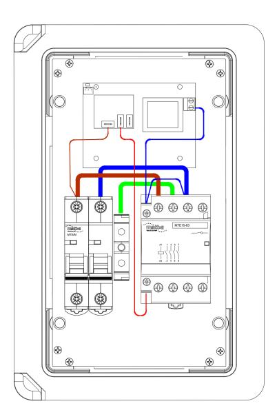
Connect the supply cable from the distribution board directly to the MCB 'mains in' terminals. Connect the outgoing cable to the contactor N, E, & L terminals. If required, connect the CT to the 3 pin connector on the PCB. Check <u>ALL</u> power and earth connections before switching on.
