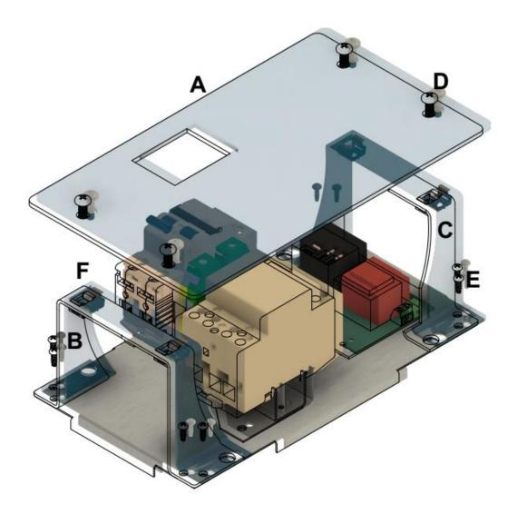
A = Touch Plate B = Touch Plate Support C = Touch Plate Support With Cut Out D = 4 No. M5x12 Screws E = 8 No. 10x10mm Screws F = 4 No. M5 Cage Nut
