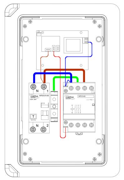
Connect the supply cable from the distribution board directly to the RCBO 'mains in' terminals. Connect the outgoing cable to the contactor N, E, & L terminals. If required, connect the CT to the 3 pin connector on the PCB. Check <u>ALL</u> power and earth connections before switching on.
