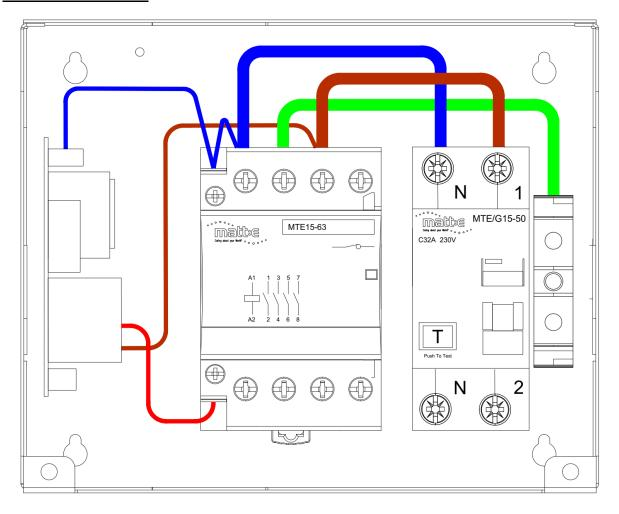
Connect the supply cable from the distribution board (or meter tails) directly to the RCBO 'Incoming Supply' terminals. Connect the outgoing cable to the contactor L, E & N terminals. If required, connect the CT to the 3 pin connector on the PCB. Check ALL power and earth connections before switching on.
