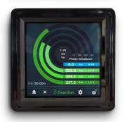
Monitoring of phase imbalances exceeding 3%, with actionable insights to optimize electrical installations and alerts viewable via the portal.
