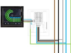
Guardian connected to the main incoming electrical supply to the building monitoring for faults that may occur on the suppliers network.
