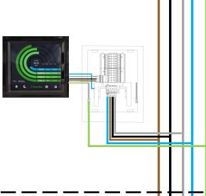
Additional Guardian devices connected at each sub distribution board helps to pinpoint the location of further faults within the electrical installation
